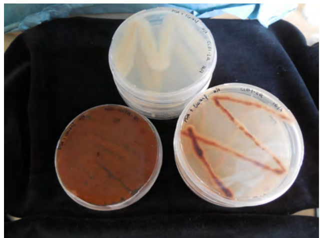
Figure 14.7 Inoculated colonies from growing plates corresponding to the file cabinet after five days on potato dextrose agar. Claudia Barra
