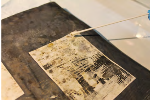
Figure 14.4 Taking a microbiological sample from the photographic album with a swab. Natalia Boero
