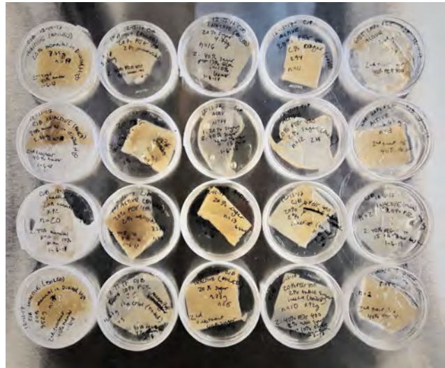
Figure 5.6 Array of bacterial cellulose samples in petri dishes during immersion solution treatment. © Courtney Books, Speculative Life Biolab, Concordia University, Montreal, 2018
